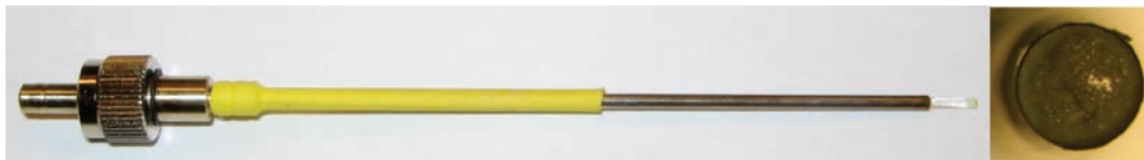
Figure 1. (Left) Fiber optic probe (actual size) used for dissolved O 2 sensing. (Right) Tip of fiber optic with compound at 50× magnification.
